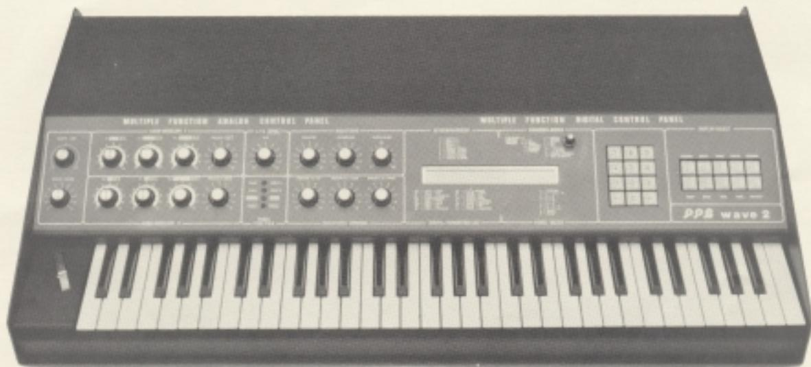
A problem with previous programmable synthesizers is that once a sound has been committed to the synthesizer's memory and the controls changed, it is impossible to see how the sound was made. For this reason, the „Wave 2“ provides an eighty character LCD (liquid crystal display) which shows information of all control settings. A numeric keyboard is also provided, which, in conjunction with the display, can be used to update and change the preset sounds.
