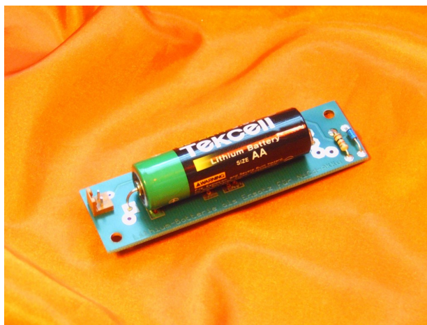
Special lithium cell with additional protective (Connection cable with plug not shown)
